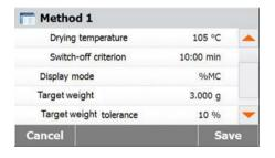
Press **Target weight tolerance** to set the tolerance of target weight.
