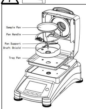
Open the cover and remove the pan handle, sample pan, draft shield, and heat shield from the instrument before cleaning.
