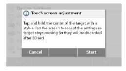
Press Touch screen adjustment to adjust the touch screen. Press the Start button to start the
