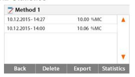
Select the method name to list all the test results of the method.
