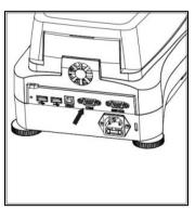
**Attention:** The RS232 port (COM 1) is located near the USB device port.
