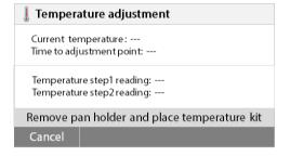
You are now prompted to remove the pan support. Place a temperature calibration kit and close the upper housing.
