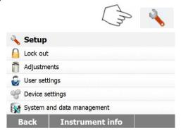
Press Setup button to access the Setup menu.
