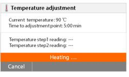
The dryer unit is heated to a temperature of 100°C. You can observe the progress on the display as the dryer temperature and count down period are displayed. After 15 minutes, read the thermometer through the inspection window on the cover and enter this temperature. Adjust the display reading to agree with the thermometer, then press the **Enter** button. You have 15 minutes to make this adjustment, otherwise the adjustment is terminated.
