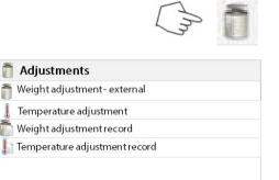
Press the Adjustment button to access adjustment menu.
