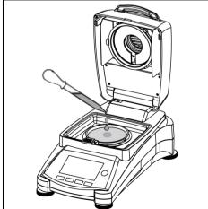
Wet the glass fiber pan with a 0.5 to 1 gram of water. Attention: Minimum sample size must be greater than 0.5 gram.
