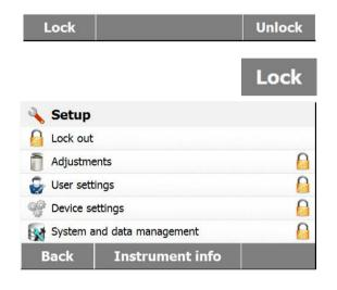
Press **Lock** to lock out Press **Unlock** to release.
