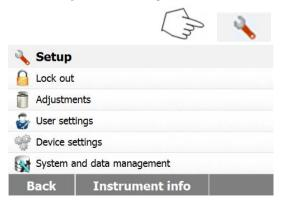
Press Setup button to access the Setup menu.
