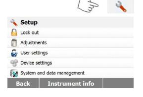
Press Setup button to access the adjustment menu.
